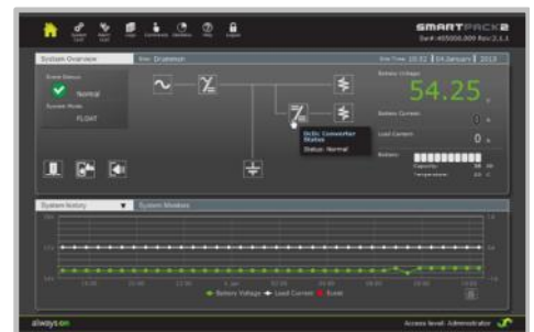
STATUS OF DC/DC CONVERTERS IN SMARTPACK2 WEB
