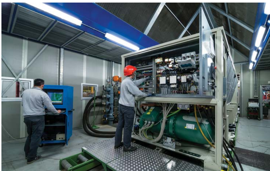
Witness test cabins have been designed to optimize the reliability of unit testing, ensuring that real installation conditions are simulated in order to confirm the unit's guaranteed performance.
