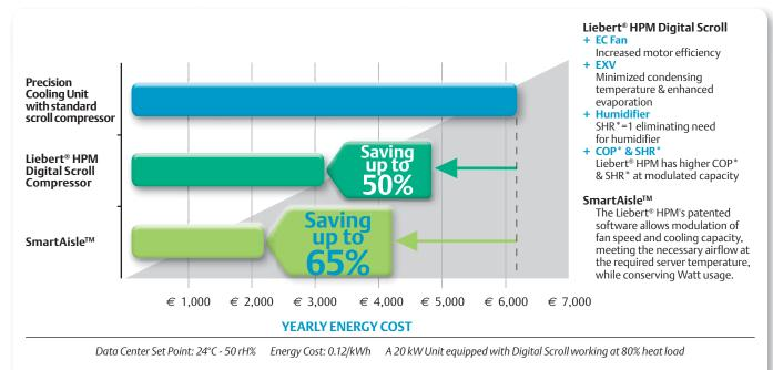
Annual savings achieved by the Liebert<sup>®</sup> HPM, complete with the most advanced technologies in the market (Digital Scroll Compressor, Electronic Expansion Valve, EC Fan) as standalone and integrated with cold aisle containment, compared to Precision Cooling units fitted with standard scroll.
