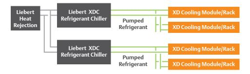
The indoor Liebert XDC Refrigerant Chiller is specifically designed to support Liebert XD cooling modules. Liebert connects directly to the modules through the pumped refrigerant circuit.
