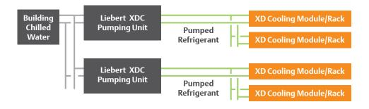
When a building chilled water circuit is available, the Liebert XDP Pumping Unit is utilized as an interface between the pumped refrigerant circuit and the chilled water system. Both Liebert XDC and Liebert XDP units circulate the refrigerant to the Liebert XD modules, while maintaining the refrigerant at a temperature always above the actual dewpoint.
