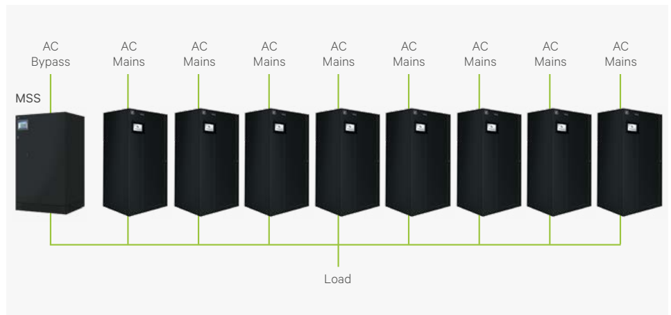
Liebert EXL centralized parallel configuration, with MSS plus 8 UPS units in parallel
